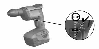
The tool is equipped with a switch safety lock that can be used to lock the control switch, thereby preventing inadvertent starting.
