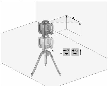
Press the +/- buttons on the laser receiver or the arrow buttons on the PRA 90 to shift the horizontal plane up or down (parallel).
