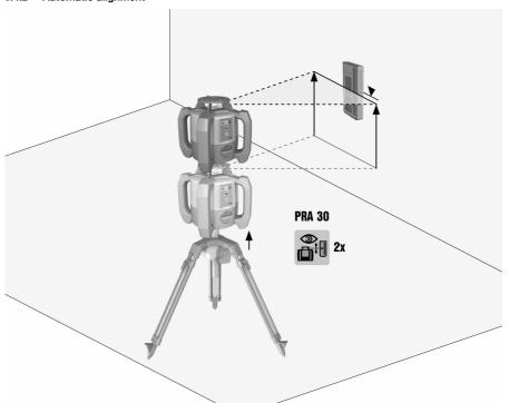
Keep the receiver side of the laser receiver at the desired target height and towards the PRA 90 control
