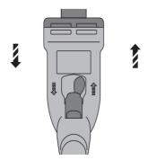
• Set the forward / reverse selector switch to forward or reverse rotation.
