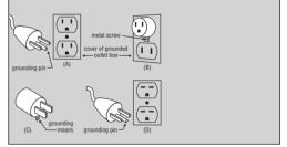
**26. Extension Cords.** Use only 3-wire extension cords that have 3-prong grounding-type plugs and 3-pole receptacles that accept the tool's plug. Replace or repair damaged cords.
