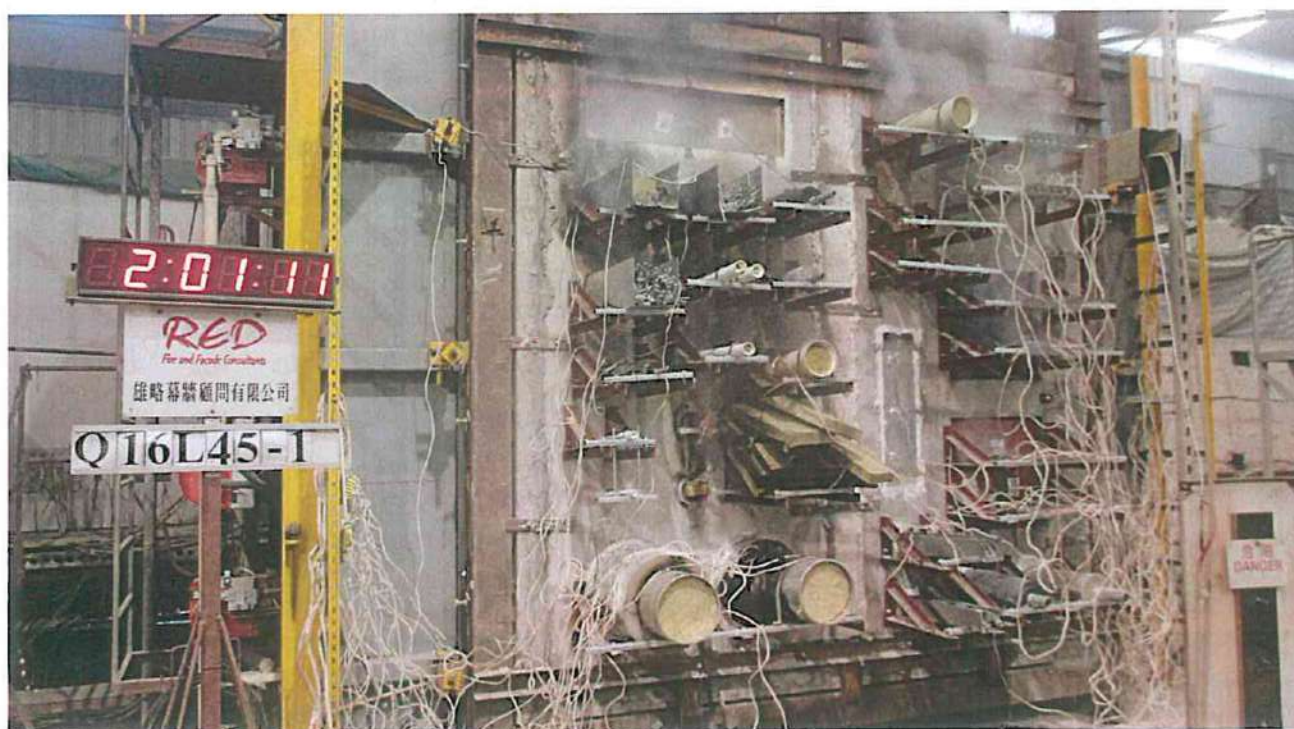
Photo 5: The unexposed face of the specimens after the test.
